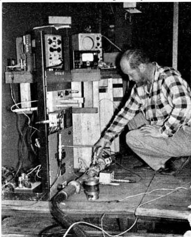
Inside the tent at W1BU. Left, the 1 kW klystron 1296 Mc/s amplifier; right, W1FZJ tunes up the moonbounce receiver. Both W1BU and W6HB used Microwave Associates MA2-1000 parametric amplifiers in their 1296 Mc/s receivers.
