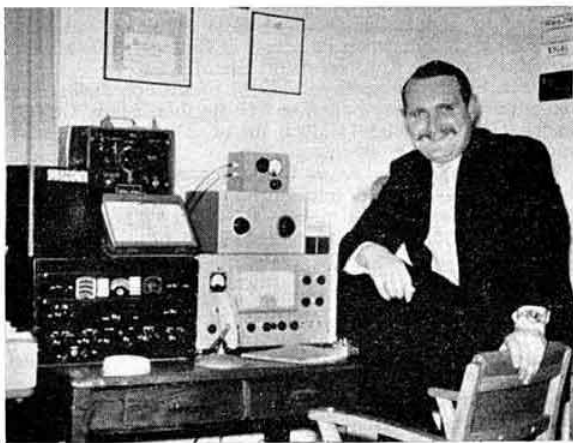
Gordon Moore was licensed as G3MCY in 1957 and now operates from R.A.F. Tangmere, near Chichester. Equipment shown in this picture includes an RCA-AR88D receiver, a BC221 frequency meter and a KW Vanguard transmitter, surmounted by a Z Match aerial tuning unit and a "Mickey Match" s.w.r. indicator. Aerials in use are a G5RV, a 15m dipole and a dipole for Top Band 60 ft. high. The main interest is county chasing on Top Band. G3MCY is an exile (albeit voluntary!) from north of the Tartan Curtain and is keen to arrange skeds with GM stations.
